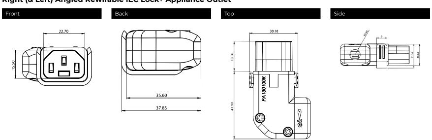
All dimensions in mm; 1 inch = 25.4 mm Tolerances according: ISO 2768-m/EN 22768-m
